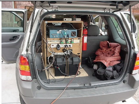
Rear view of rack with deep cycle battery & pump system feeding the analyzers.
