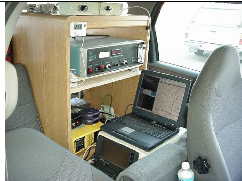
View looking from front seat to the back instrument rack, inverter & computers.
