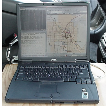
Display on front seat computer for CO concentration, vehicle position and observation log entry.
