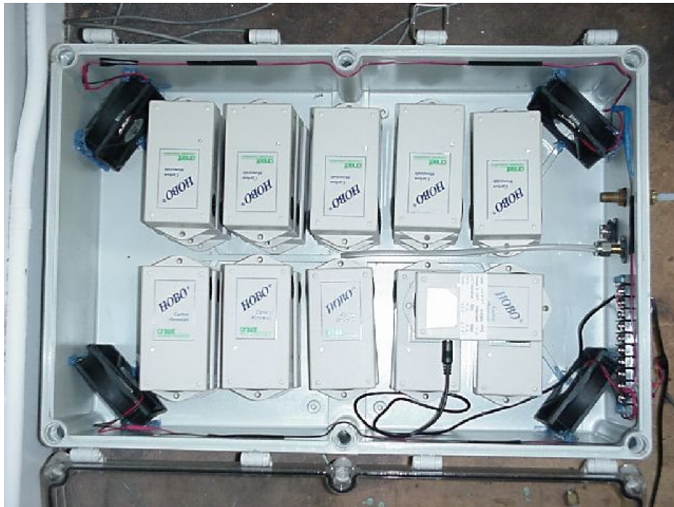
Figure 4-1. Chamber for Calibrating the Onset CO Analyzers
