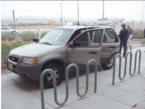
Sampling Van (sample inlet & temperature probe were on roof-mounted antenna)
