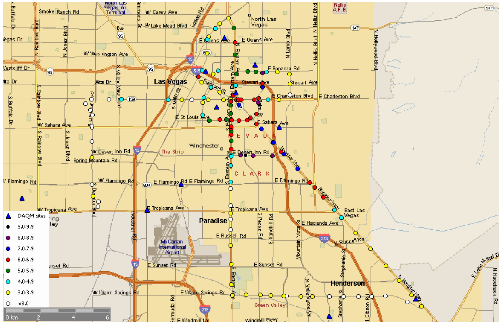
Figure 6-8. Observed CO Concentrations (ppm) During December 17 Morning Period
